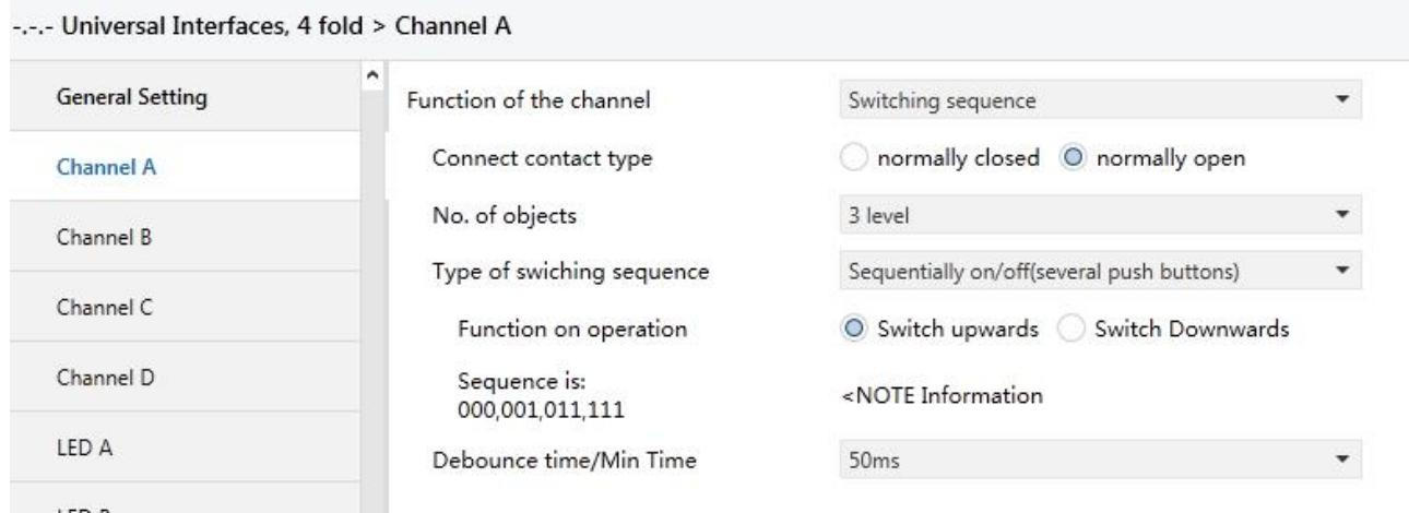
Fig.11 Parameter window “switching sequence, X”
